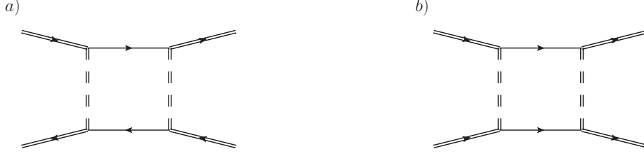
Figure 2: Additional diagrams for F\bar{F} and FF annihilations induced by the Yukawa interaction. Solid double lines stand for F , solid thin line for the SM quark and double dashed line for the scalar DM. The colour flux is different from the diagrams induced by QCD.
