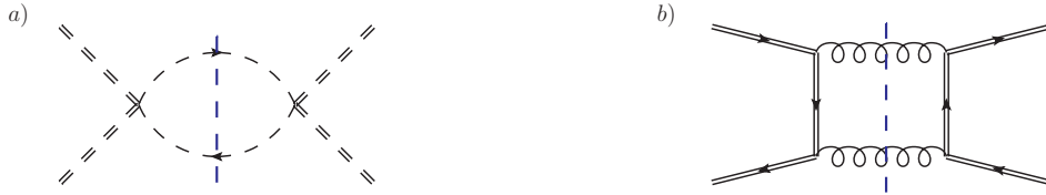
Figure 1: One-loop diagrams for DM pair (double-dashed lines) annihilations into SM Higgs bosons (dashed lines) and F\bar{F} (double-solid lines) annihilations into a gluon pair (curly lines). The blue dashed line implements a cut along the light particles into which the heavy ones annihilate.
