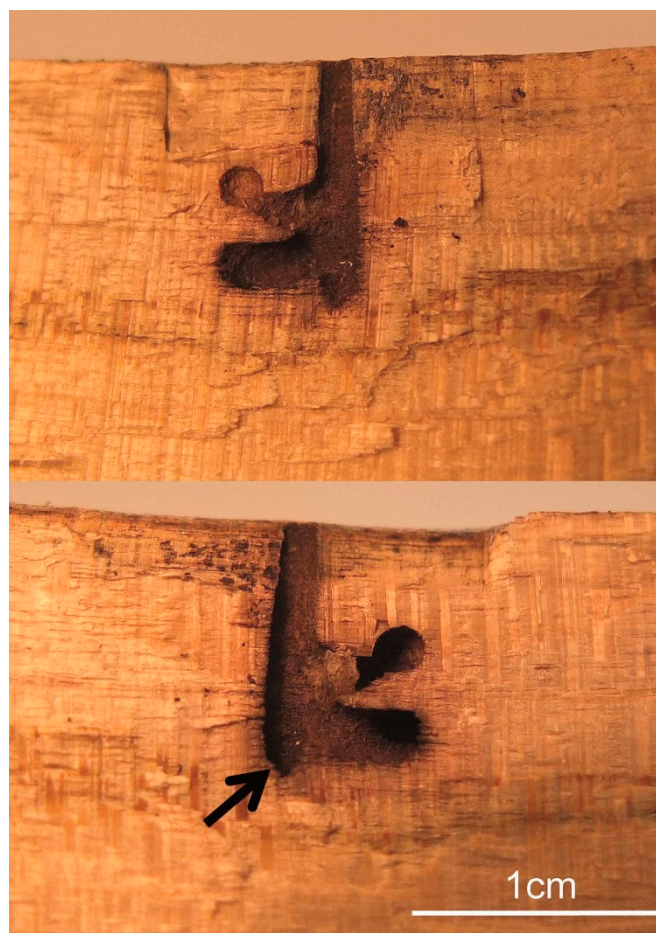
Figure 7. Example of the entrance to an insect gallery of Xylosandrus germanus cf. The dark color of the gallery was caused by an Ambrosia fungus, which the beetle established as food-source in the tunnel. The black arrow indicates the continuation of the tunnel following the annual ring.
