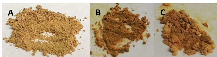
Figure S7. Fresh CN-OA-m (A), CN-OA-m after 8 h white light irradiation for standard reaction (B) and CN-OA-m after 48 h green light irradiation for standard reaction (C).
