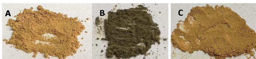
Figure S8. Fresh CN-OA-m (A), CN-OA-m after recyclability tests with white light irradiation (B) and CN-OA-m after recyclability tests with green light irradiation (C).
