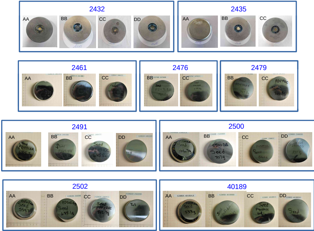
Fig. 1 Full inventory of crystal slices / diodes belonging to the GERDA Phase II BEGe detector production. Crystals / diodes obtained from the same ingot are framed in blue. The GD32 and GD35 detector series belonging to the 1 st batch are depicted in their final diode form (row 1), while the other 7 series from the 2 nd batch are shown as crystal slices prior to diode conversion (rows 2 to 4).
