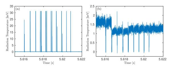
**Figure 5.13** – Degradation of ECE mixer during a rotating magnetic island in ASDEX Upgrade #35939. Pane (a) shows the signal from a channel around 75.5 GHz; pane (b) shows the signal from a channel around 87.9 GHz.
