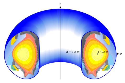
**Figure 1.1** – Schematic cross section of ASDEX Upgrade illustrating the main parameters and plasma shape in the divertor configuration. Picture is adapted from the ASDEX Upgrade drawing gallery [40].
