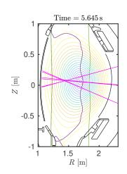
**Figure 5.24** – Plasma scenario with central PDIs in ASDEX Upgrade #36149. Green lines are ECR harmonics, magenta lines are gyrotron beams, and purple lines are the 70 GHz warm UHR.
