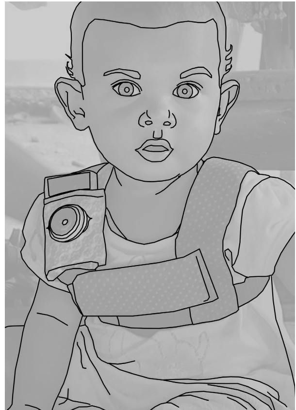
Figure 1. The recording vest included an Olympus audio recorder in the front horizontal pocket and a miniature camera with a fish-eye lens on the shoulder strap.
