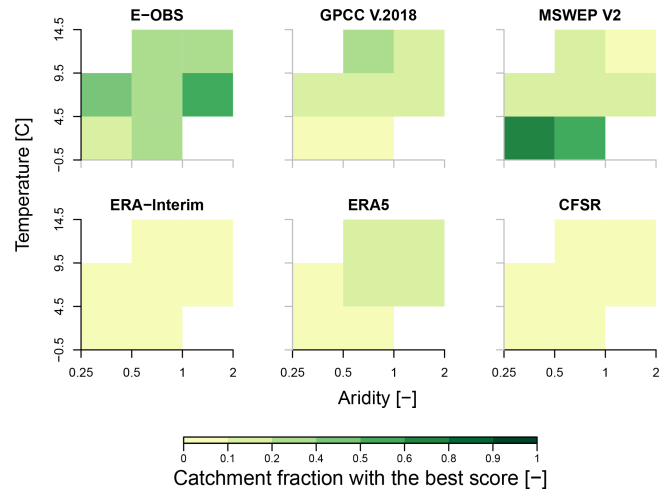
Figure 6. Runoff-based performance of precipitation products across climate regimes. Colors refer to the percentage of catchments within each box recognized as the best performance based on anomaly correlation and absolute bias during May–September.
