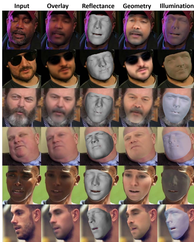
Figure 10. Limitations of our approach. From top to bottom: Extreme illumination conditions, severe occlusions by accessories, thick facial hair, non-average facial shapes, scale ambiguity between illumination and reflectance, and extreme head poses.
