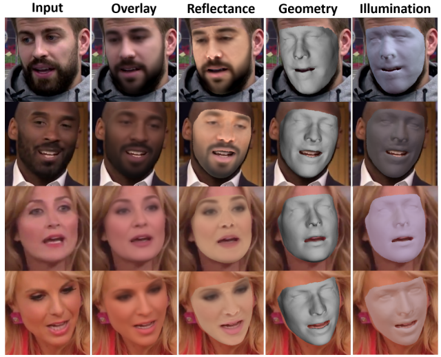
Figure 4. Our approach produces high-quality monocular reconstructions of facial geometry, reflectance and illumination by learning an optimal model from in-the-wild data. This enables us to also reconstruct facial hair and makeup.
