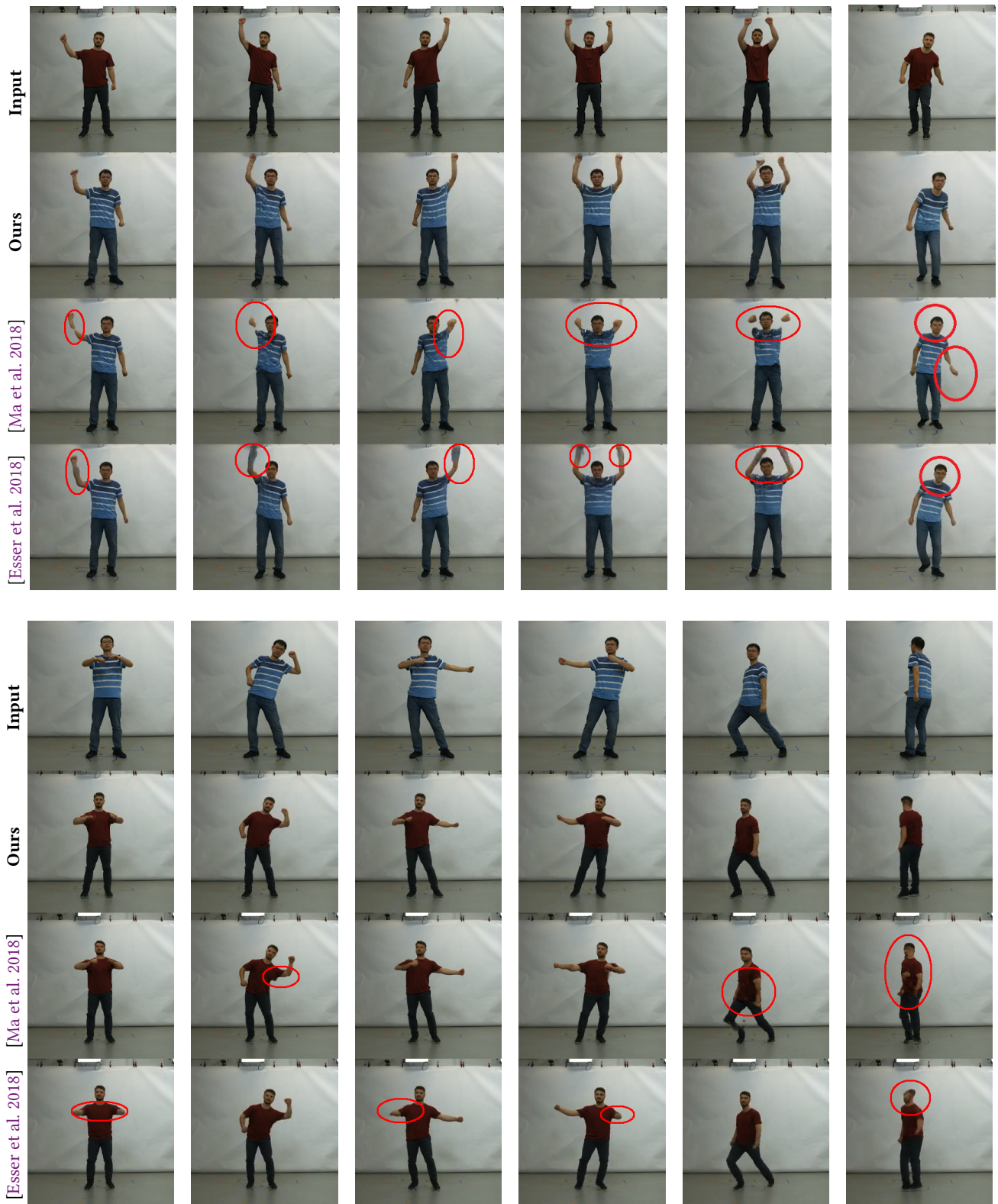
Fig. 6. Qualitative re-targeting comparison of our approach to the state-of-the-art human image synthesis methods of Ma et al. [2018] and Esser et al. [2018]. The encircled areas show regions of the body where the other methods clearly fail (missing parts of arms, wrongly shaped body parts etc.) in comparison to our approach. For the full results we refer to the supplementary video.
