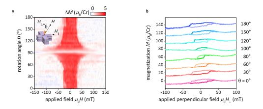
**Figure 5** | **Monolayer CrBr**<sub>3</sub> in tilted magnetic field. a, Angular dependence of the amplitude of the magnetic hysteresis  $\Delta M$  as a function of H and  $\theta$ . Inset: Our rotation setup is shown schematically. b, Hysteresis loops as a function of  $H_{\perp}$  for several angles.
