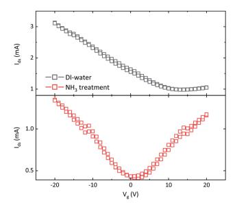
Fig. 2 Transfer characteristics of FETs fabricated with graphene layers that are washed only in DI-water (top) and DI-water plus aqueous ammonia flow (bottom). Both transistors have channel length and width of 10 and 1000  $\mu$ m, respectively. The bias on drain electrode is +100 mV. Source electrode is grounded.
