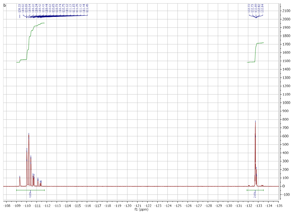
Figure S1-c. ^{19}\text{F} -NMR (367 MHz) spectrum of b in \text{CDCl}_3
