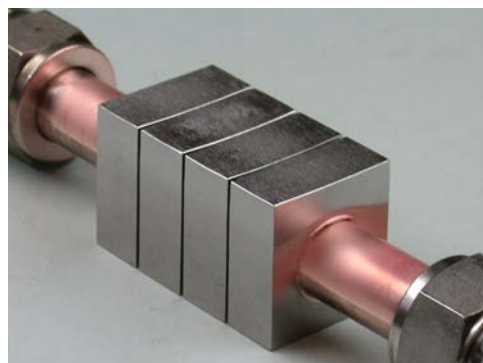
Fig. 1: Example of a HHF tested W monoblock mock-up. The mock-up is equipped with 23 \times 12 \times 28 \text{ mm}^3 W blocks provided by A.L.M.T (JP) or AM&T (CN).
