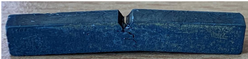
Figure 4 typical porous matrix W_f/W after the 3-point bending test
