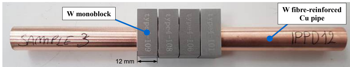
Figure 7. Monoblock type PFC mock-up with W f -Cu MMC heat sink pipe before HHF loading.
