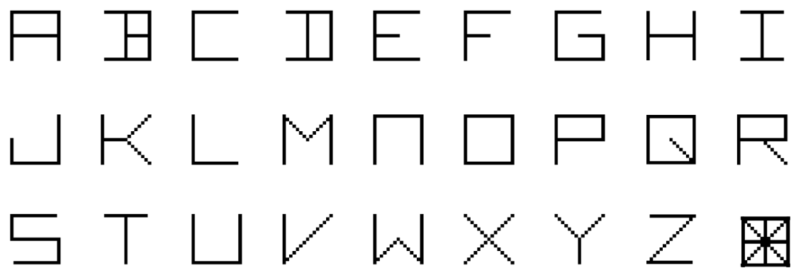
Supplementary Figure 12 Illustration of virtual font. Illustration of the virtual font presented to the network. In this font all 36 alphanumeric characters can be formed from only 14 line segments. This allows each character to be encoded as a 14-dimensional input vector representing visual features. Font is adapted from Rumelhart and Siple 3 , slightly modified to increase similarity between U and N, and overlap with other letters, as we used in our experiment.
