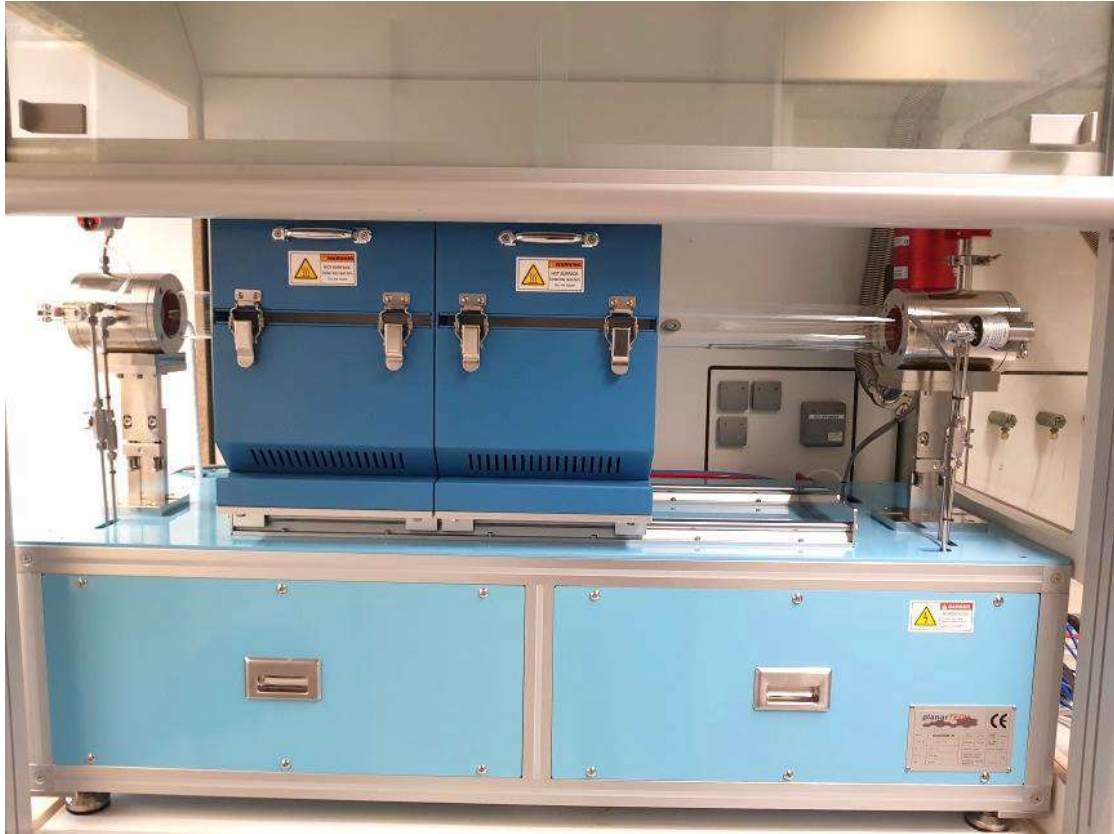
Figure 2.4. CVD setup PlanarGROW 3S, from PlanarTech, used in this work.
