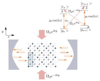
Figure 1. Geometry sketch to realize a dynamical version of the Harper-Hofstadter Hamiltonian: a 2D Fermi gas in a rectangular lattice within a single-mode optical cavity is transversely illuminated by two counter-propagating laser beams of orthogonal polarization. The shaded area in the lattice represents the unit cell for  $\phi = 2\pi/3$ .
