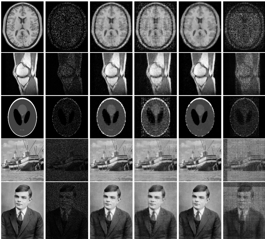
Fig. 8. Comparison of image recovery by using different techniques when 20% data are observed with some noise (PSNR = 20). From the left to the right in each row: original image, observed image, the recovered image by IRNN.TV, IRNN, TFOCS, and LMaFit, respectively
