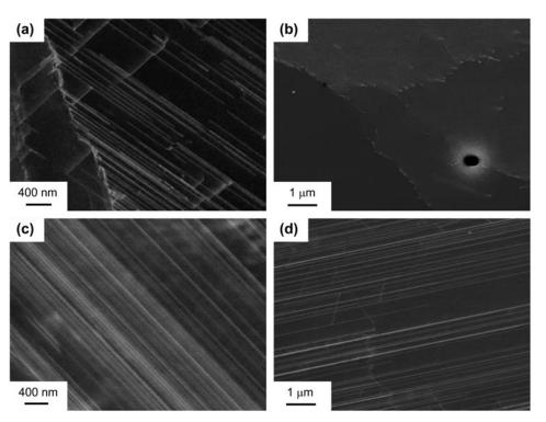
Figure 3: ECC images of (a) C15 NbCo<sub>2</sub> at 25.6 at.% Nb, (b) C15 NbCo<sub>2</sub> at 30 at.% Nb, (c) C36 NbCo<sub>2</sub> at 25.1 at.% Nb, and (d) C14 NbCo<sub>2</sub> at 36 at.% Nb taken from the NbCo<sub>2</sub> alloys.
