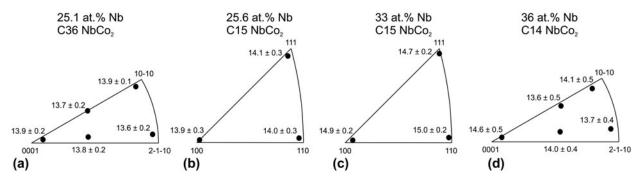
Figure 6: Hardness of (a) C36 NbCo2 at 25.1 at.% Nb, (b) C15 NbCo2 at 25.6 at.% Nb, (c) C15 NbCo2 at 33 at.% Nb, and (d) C14 NbCo2 at 36 at.% Nb measured from the NbCo2 alloys in various orientations.
