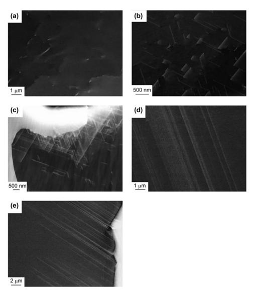
Figure 2: ECC images of (a) C15 NbCo<sub>2</sub> at 30 at.% Nb, (b) C15 NbCo<sub>2</sub> at 25 at.% Nb (Co-rich phase boundary), (c) C15 NbCo<sub>2</sub> at 34.3 at.% Nb (Nb-rich phase boundary), (d) C36 NbCo<sub>2</sub> at 24.5 at.% Nb, and (e) C14 NbCo<sub>2</sub> at 36 at.% Nb taken from the diffusion couples.
