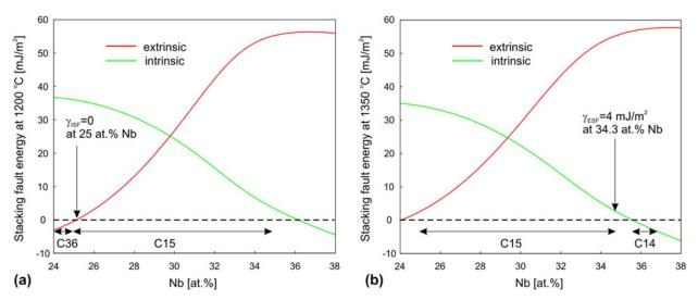
Figure 8: Calculated intrinsic (i.e., C14-like) and extrinsic (i.e., C36-like) SFE of the C15 NbCo<sub>2</sub> Laves phase at (a) 1200 °C and (b) 1350 °C as a function of composition.
