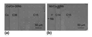
Figure 4: SEM images showing the indents in the diffusion zones of the cubic and hexagonal NbCo2 Laves phases in the diffusion couples (a) Co/Co-30Nb and (b) Nb/Co-30Nb.
