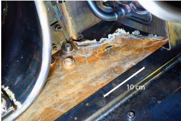
Fig. 2 The Status of the vessel after the opening. A stainless steel protection at the low field side midplane is shown. The white crystals are borate, brownish layers are rust.
