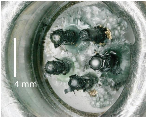
Fig. 4 Electrical feed through with Mo pins. The white crystals are Molybdenum Oxides, remnants of the Au plating are also found.
