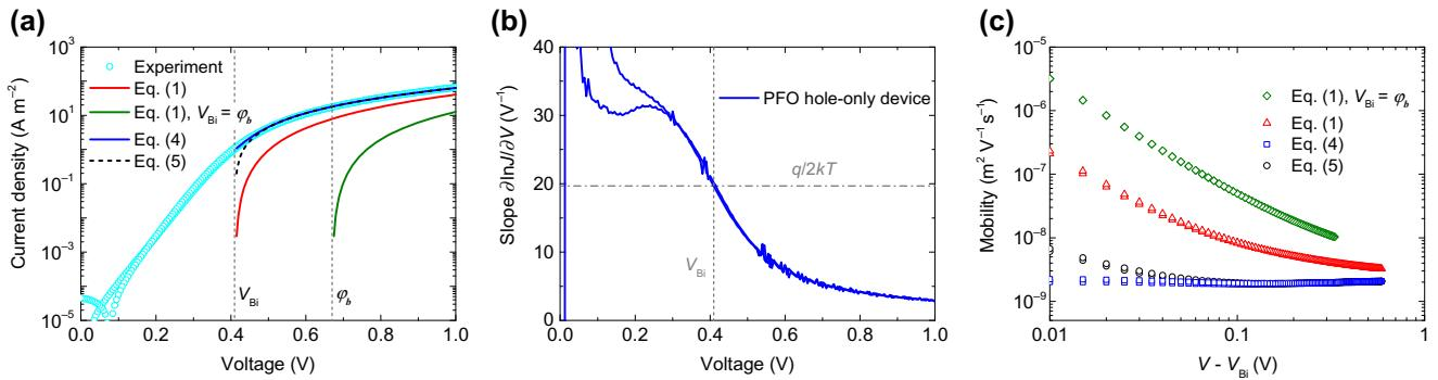
FIG. 4. (a) Experimental  $J$ - $V$  characteristic of a PFO hole-only device (symbols) and calculated  $J$ - $V$  characteristics above  $V_{\text{BI}}$  (vertical dashed lines), with the green line calculated for  $V_{\text{BI}} = \varphi_b$ , neglecting band bending. (b) Derivative of the experimental  $J$ - $V$  characteristic, indicating the built-in voltage (vertical dashed line). (c) Hole mobility extracted with different equations.
