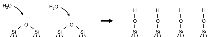
Figure 6. Recovery of surface silanols on silicon oxide via dissociative adsorption of water.
