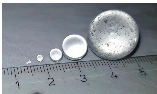
Fig. 3. Transparent glass beads of different size ranging from 0.4 mm to 16 mm mimicking fine sand and coarse aggregates.
