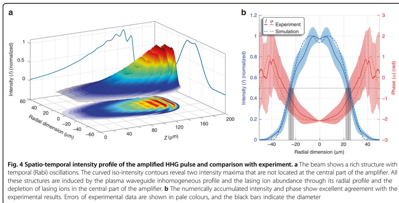
resulting in the two-peak profile and the phase that the experiment revealed is in excellent agreement with the simulation, as shown in Fig. 4b.
