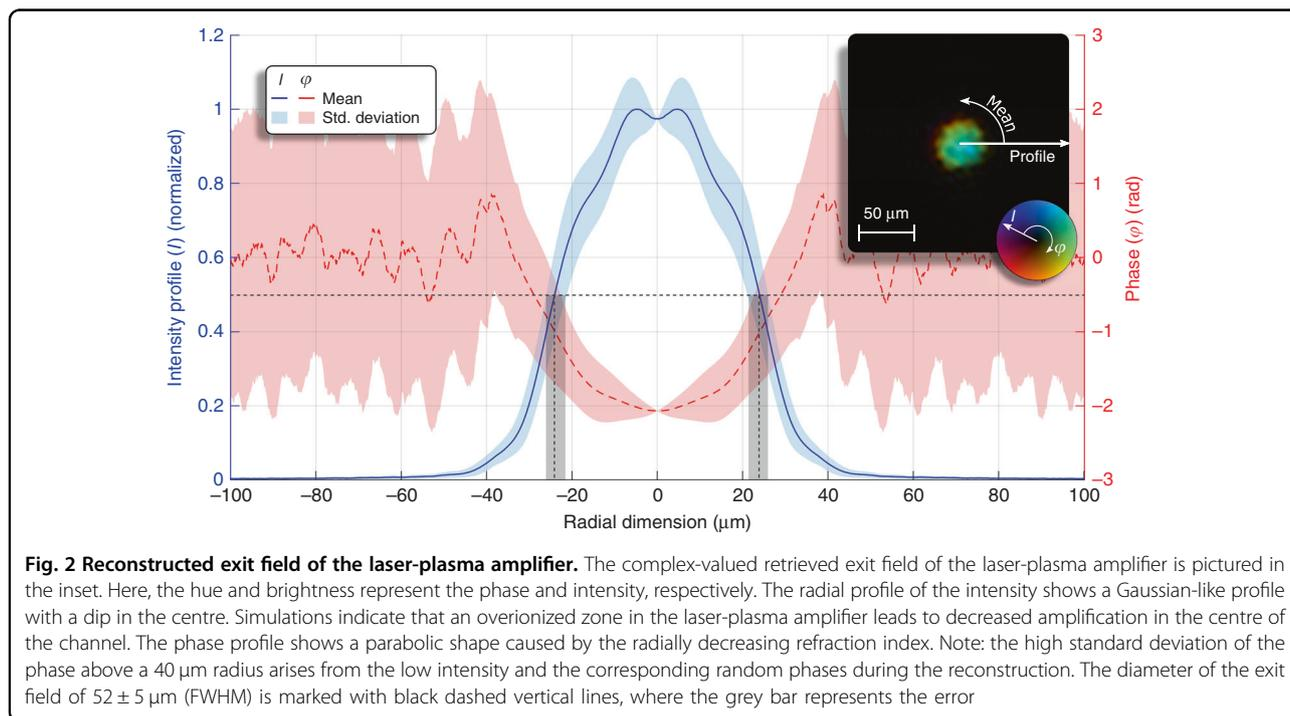
accordingly. The increased standard deviation of the phase for larger radii emerges from the near-zero intensity due to the reconstruction process and the consequently random phases.
