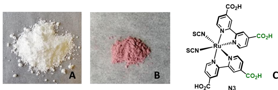
Fig. S7. N3-TiO 2 -NiCl 2 ·dcbpy. Unfunctionalized TiO 2 Aeroxide P25 (A) and N3-TiO 2 -NiCl 2 ·dcbpy (B). Structure of N3 (C). The functionalities that bind to the surface hydroxyl groups of TiO 2 are marked in green.
