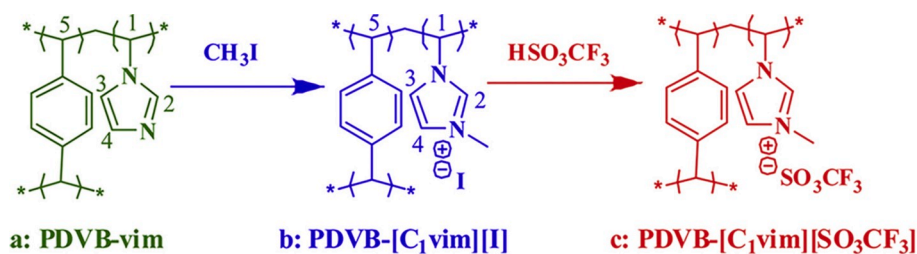
Fig. 5. The synthetic scheme for the preparation of PDVB-[C 1 vim][SO 3 CF 3 ] from PDVB-vim [52]. Copyright 2012, American Chemical Society.
