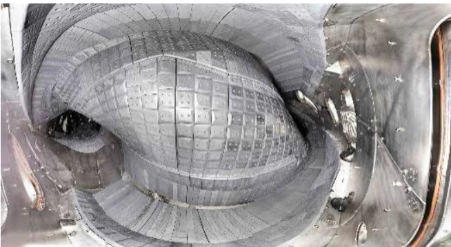
Fig. 6. Fish eye view in the plasma vessel with the completed TDU. Below in the middle of the photograph one sees horizontal and vertical target modules with the sickle-shaped pumping gap in between.
