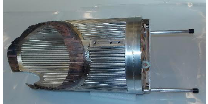
Fig. 8. Actively cooled port liners protect the port wall from heat radiation of the plasma (courtesy NTG Neue Technologien GmbH)
