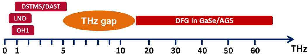
**Figure 2.7. General table-top techniques of intense THz pulses generation.** Below 5 THz, Optical rectification are widely used in ferroelectric material (e.g. LiNbO<sub>3</sub>) and large piece of organic crystals (OH1, DSTMS, DAST). Above 15 THz, frequency mixing using near-infrared pulses can be exploited in semiconductor emitters like GaSe, AgGaS<sub>2</sub>. Efficient light source in the “THz gap” is still on demand.
