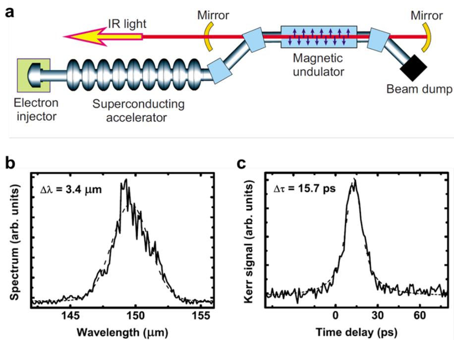
**Figure 2.1.** (a) Schematic view of the free-electron laser in the FZD. (b) Measured spectrum of the FEL at 150- $\mu\text{m}$  wavelength. (c) The Electro-optic sampling of the free electron laser pulses in a ZnTe crystal. The FWHM of the Kerr signal reveals a pulse duration of  $\sim 16$  ps. Taken from Ref. [40].
