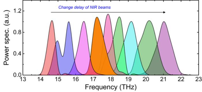
**Figure B.2** Power spectrum of the generated MIR pulses using GaSe crystal.
