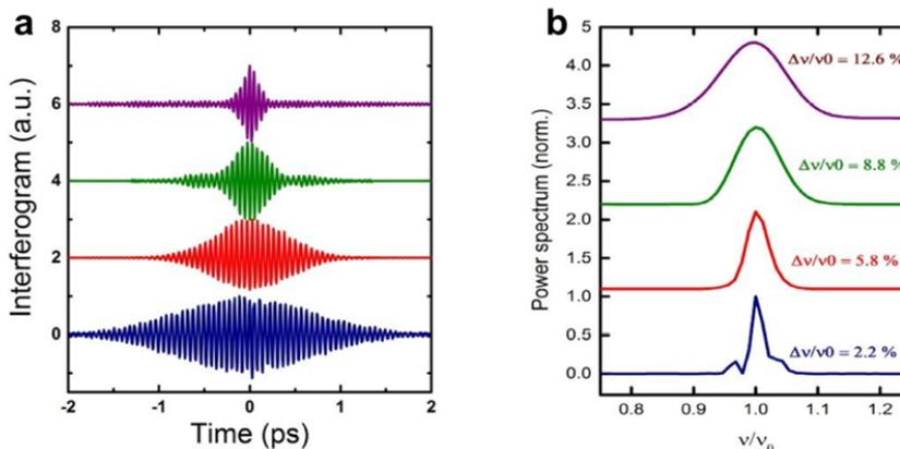
**Figure 2.18.** (a) Interferograms for the THz fields generated by using near-IR pulses with different duration. (b) The corresponding relative bandwidth  $\Delta\nu/\nu_0$  (FWHM) of the THz fields shown in (a).
