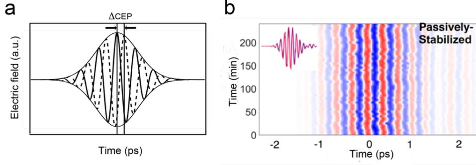
**Figure 2.19.** (a) Example of carrier-envelope phase shift. (b) CEP stability characterization of narrowband pulses. Due to the passive stabilization in the difference frequency generation process, the recorded electro-optical sampling over 240 minutes (4 hours) with negligible drift proves the generated pulses to be CEP stable. Inset: EOS traces measured with of 1-hour interval.
