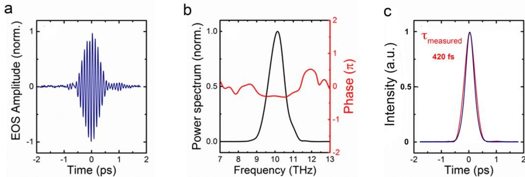
**Figure 2.15.** (a) The THz electric field generated by DFG in a 480  $\mu\text{m}$  thick DSTMS crystal as detected via electro-optic sampling in a GaSe crystal of 100  $\mu\text{m}$  thickness. (b) Corresponding power spectrum (black) and spectral phase (red). (c) Retrieved pulse duration from the EOS measurement (red) and the constructed transform limit pulse from the measurement (blue).
