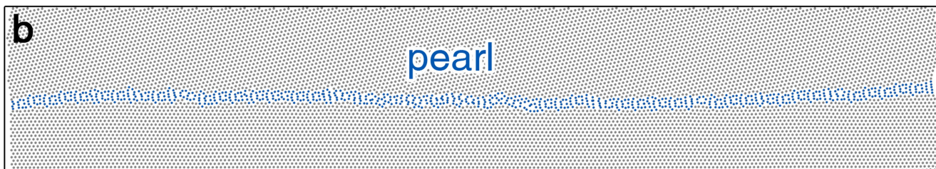
Extended Data Fig. 5 | Asymmetric GB transformation at 600 K. a, Nucleation of a pearl GB phase at the open surface (left) of the asymmetric GB at 600 K. b, Asymmetric pearl GB phase after the transformation at 600 K is complete. The boundary remains asymmetric.
