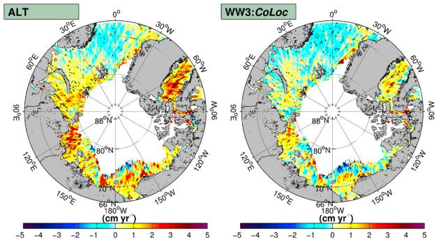
Fig. 9. Trends of monthly averaged significant wave height ( $H_s$ ) datasets (cm yr<sup>-1</sup>) with the Mann–Kendall test (thatched areas) from (left) satellite altimetry (ALT), and (right) collocated model WW3 hindcast (CoLoc).
