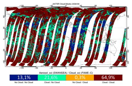
Fig. 4. Consistency overview between Aerosol\_cci (Swansea University) and Cloud\_cci (FAME-C) AATSR cloud masks for observations of four selected days in September 2008. "No cloud/no cloud" and "cloud/cloud" situations are solely analyzed as aerosol or clouds in Aerosol\_cci and Cloud\_cci, respectively. "No cloud/cloud" situations are wrongly analyzed as aerosols and clouds, while "cloud/no cloud" situations are not analyzed at all.
