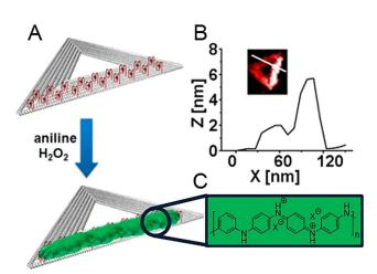
**Figure 4.** A) DNA-templated synthesis of polyaniline (green) on origami triangles (gray) with DNAzymes (red structures with black dots) in the presence of aniline and  $H_2O_2$ . B) AFM image of a single PANI-coated origami triangle. C) Structure of the emeraldine salt form of PANI. Reprinted from Ref. [26] with permission; Copyright (2020) American Chemical Society.
