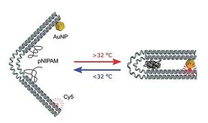
Figure 12. Representation of the DNA origami flexor. Upon heating of the flexor-containing solution, PNIPAM aggregates and leads to a change in the DNA origami shape. Reprinted from Ref. [39] with permission.
