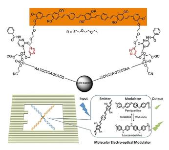
Figure 8. Top: Product of the double-CuAAC reaction between an azide-functionalized oligomer (OPV) and an alkyne-functionalized oligonucleotide sequence, immobilized on a solid support (controlled pore glass). Bottom: Schematic representation of the x-shaped OANI-and OPV-DNA conjugate on the DNA origami frame. OANI (blue) acts as a modulator of the fluorescence intensity of the OPV (orange). Reprinted from Ref. [37] with permission. Copyright (2020) American Chemical Society.
