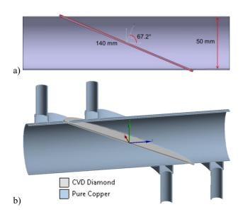
Fig. 1. Diamond Brewster window (a) and a conceptual cooling layout (b) to remove the heat absorbed in the disk.
