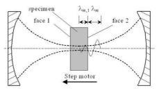
Fig. 5. Spherical Fabry-Perot resonator consisting of two spherical mirrors and the disk placed at the center. It allows high resolution measurements of tan $\delta$  at the center of the disk.
