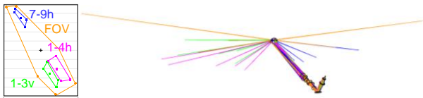
Fig. 4: Sequential Zemax model with 4 configurations: Footprint on sensor (left), lines of sight from divertor to sensor (right)
