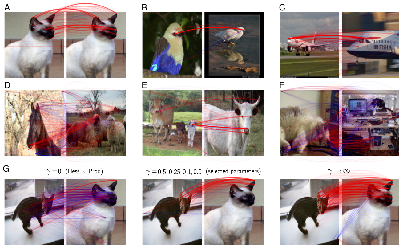
Fig. 6. Application of BiLRP to a dot-product similarity model built on VGG-16 features at layer 31. Top : BiLRP explanations on different pairs of input images from the Pascal VOC 2007 dataset. Red and blue color indicate positive and negative contributions to the similarity. (Details of the rendering procedure are given in Appendix E of the Supplement.) Bottom : Effect of the BiLRP parameter \gamma on the explanation.
