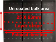
Figure 2. Sample measured by LIBS, (a) location of the samples, (b) layered structure of the sample, the top C layer is 5-10 \mu\text{m} , the C/Mo coexistence layer is about 3.2 \mu\text{m} (c) image of one sample and the laser craters.
