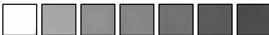
Figure 1: Sulfide images, exposed to 0.3 mM di-sodium-sulfide solution for calibration after 0, 0.15, 1, 2, 6, 12 and 24 hours.
