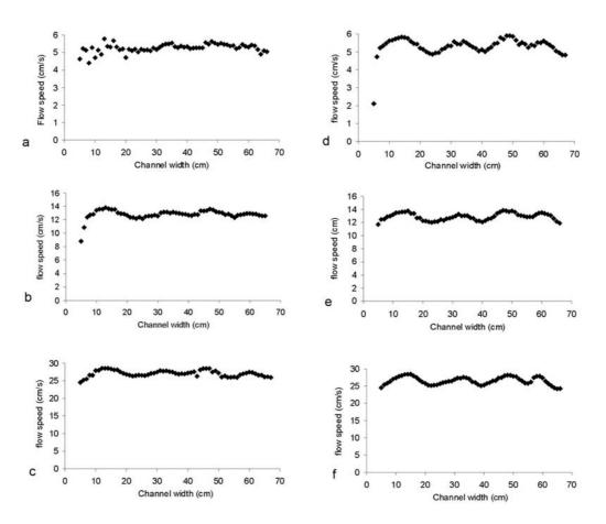
Fig. 7. The wall layer in the middle of the test section at the three stream velocities of a) 5 cm s<sup>-1</sup>, b) 12 cm s<sup>-1</sup> and c) 25 cm s<sup>-1</sup>, and sidewall effect at 230 cm ahead of the test section at stream velocities d) 5 cm s<sup>-1</sup>, b) 12 cm s<sup>-1</sup> and c) 25 cm s<sup>-1</sup>. The measurements started on the inner wall and moved towards the outside wall of the flume.
