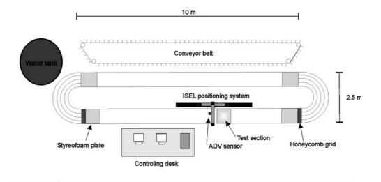
Fig. 1. The benthic flume plant at the OceanLab
