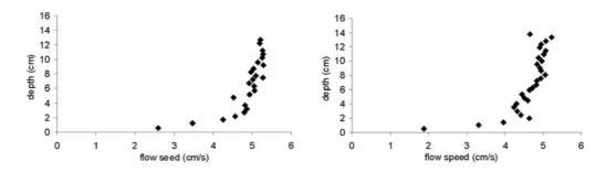
Fig. 6.Velocity profiles measured in the middle of the test section at 5 cm s<sup>-1</sup> free stream flow velocity, with a Styrofoam plate and a honeycomb grid located before the entrance of the bend of the flume to reduce disturbance.
