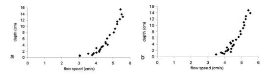
Fig. 5.Velocity profiles measured at a) 60 cm and b) 230 cm ahead the middle of the test section at 5 cm s<sup>-1</sup> free stream flow velocity.
