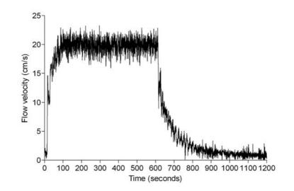
*Fig. 3.* The response time to speed changes in the centre of the flow at 11 cm from the flume bottom with a 21 cm depth water column.
