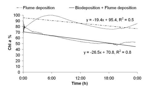
*Fig. 7:* Percentage decrease of chlorophyll a in the flume tank over time and under critical shear velocity of 0.6 cm.s<sup>-1</sup>, with sediments containing biogenic structures (solid lines) and with control sediments (dashed line).
