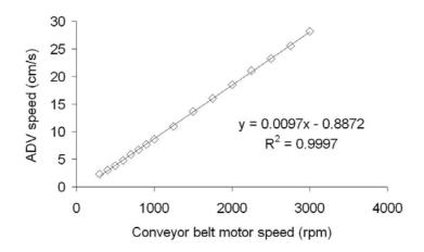
*Fig. 2. Relation between belt motor and resulting flow in the centre of the flow and at 11 cm from the flume bottom with a 21 cm depth water column.*
