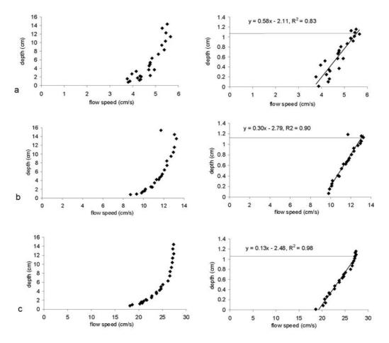
*Fig. 4. Velocity profiles (left: linear scale plot, right: semi-logarithmic scale plot) measured in the middle of the test section at three different free stream velocities (a: 5 cm s<sup>-1</sup>, b: 12 cm s<sup>-1</sup> and c: 25 cm s<sup>-1</sup>).*
