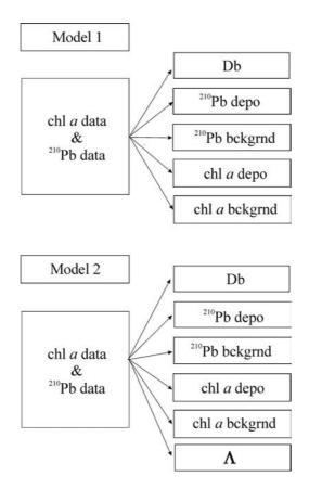
Fig. 2: Schematic representation of the model approaches (model 1 and model 2) and the derived diagenetic parameters; where Db = bioturbation rate, <sup>210</sup>Pb depo = <sup>210</sup>Pb deposition, <sup>210</sup>Pb bckgrnd = <sup>210</sup>Pb background concentration, chl a depo = chl a deposition, chl a bckgrnd = chl a background concentration, and  $\Lambda$  = the factor in Sun et al. (1993) set as 18.3 in the chl a decay relationship (Eq 4.)
