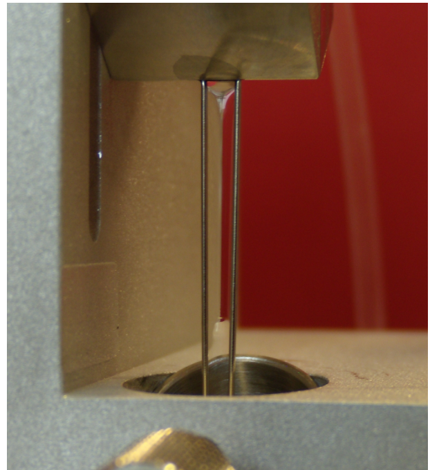
FIG. 2. View of the flowing liquid between the wires. Due to the lens in the liquid film, the wires do not appear parallel. The collector is tilted by 45° with respect to the wires.
