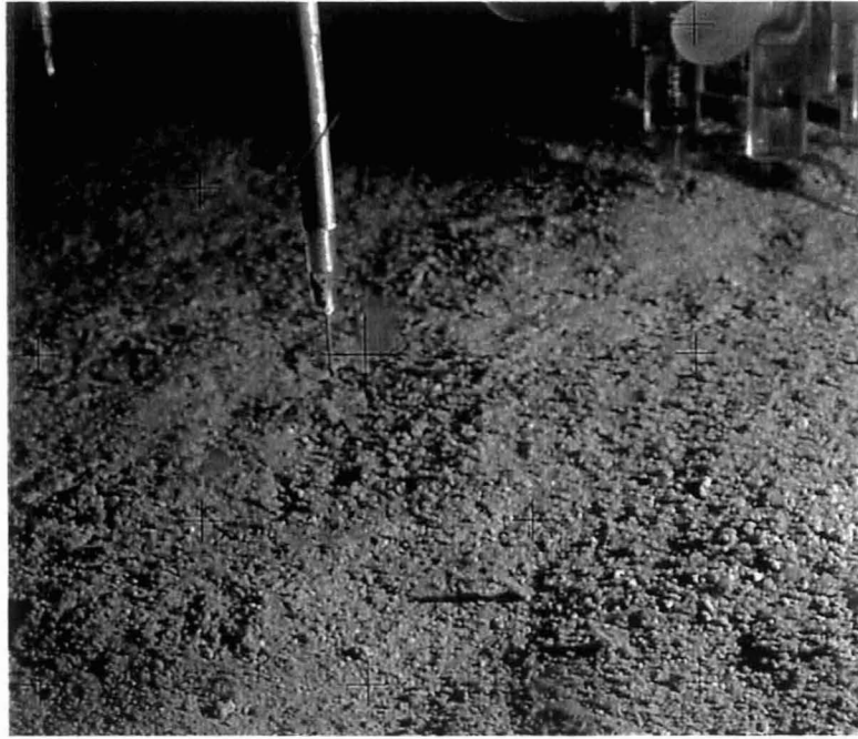
Fig. 3: Photograph of the sediment surface at GeoB 4419. Oxygen optodes can be seen in the front, while the microelectrodes penetrating across the sediment surface can be observed in the back.
