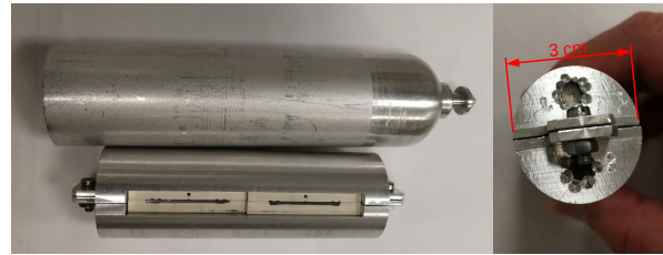
Figure 4: Irradiation rig: side view (left) and front view (right) of the custom made holders to tightly fit the sensor assemblies into the capsule (upper part on left side).
