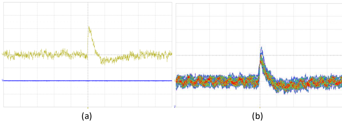
Fig 28. Output signals of version 2 board with filter, impedance decoupler and LM358 replaced with AD823 with 10M resistance and 6.8pF capacitance in the feedback loop [X-axis= 100us/div and Y-axis = 50mV/div] (a) Output signal (b) Output signal in persistence mode
