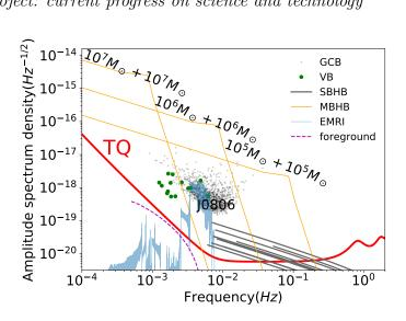
Figure 1. Expected astrophysical sources for TianQin. In this plot, the information of the detector response is included in the signal strain of each source and the instrumental noise (the solid red curve) is approximated by dividing  $S_n(f)$  by 10/3, which accounts for the geometric configuration of TianQin, as well as the location- and polarisation-sensitive response in the low frequency limit.
