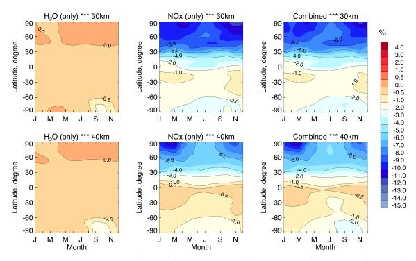
**Figure 7.** Calculated reduction in the ozone column as a function of latitude and month of the year calculated for an injection of water vapor (left panels) and nitrogen oxides (middle panels) and for the combined emissions (right panels) by the adopted HST fleet cruising at 30 km (upper panels) and 40 km (lower panels), respectively.
