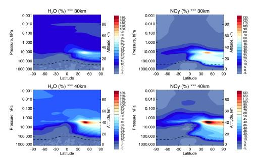
Figure 2. Annual and zonal mean perturbations (percent) in the atmospheric concentrations of  $H_2O$  (left panels) and NOy (right panels) for an injection by a fleet of HST cruising at 30 km (upper panels) and 40 km altitude (lower panels). The dashed black line is the location of the lapse rate tropopause.
