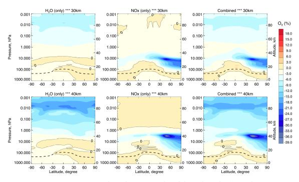
Figure 6. Percent change in the atmospheric concentration of ozone for an injection of  $H_2O$  (left panels), NOx (middle panels), and combined  $NOx + H_2O$  (right panels) by a fleet of HST operating at 30 km (upper panels) and 40 km (lower panels), respectively.
