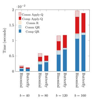
Fig. 4.1: Time breakdown for TSQR variants for  $1,024,000 \times b$  matrix over 1024 processors, including both factorization and application of the orthogonal factor to a dense  $b \times b$  matrix.
