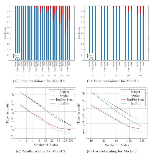
Fig. 4.3: Time breakdown and and parallel scaling of variants for TT norm computation. "Ortho" refers to orthogonalization (following by computing the norm of a single core), "InnPro" refers to using the inner product algorithm, and "InnPro-Sym" refers to using the inner product algorithm with symmetric optimization.
