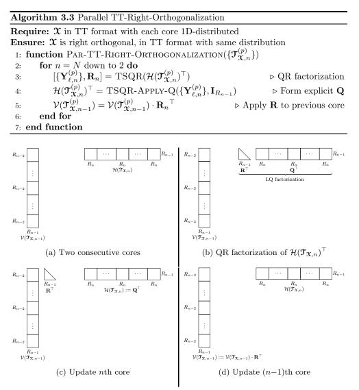
Fig. 3.2: Steps performed in TT right orthogonalization
