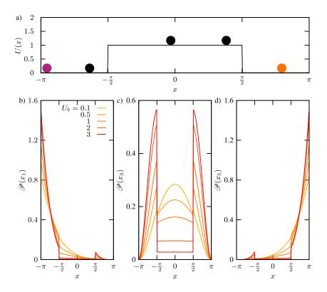
**FIG. 1.** (a) Schematic of the potential U(x) defined in Eq. (1); single file with N=5 particles. Throughout this work, we either tag the first (magenta stands for i=1) or the last (orange stands for i=1) particle. (b)–(d) depict the equilibrium probability distribution  $\mathscr{P}_{eq}(x_i)$  for i=1 (b), i=3 (c), and i=5 (d) in a single file with N=5 for different barrier-heights  $U_b$ , respectively.
