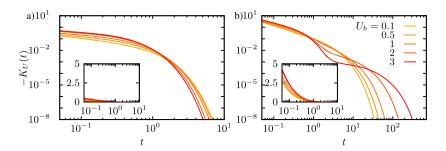
**FIG. 4.** Memory kernel  $-K_U(t)$  of an isolated particle (a) and the leftmost tagged-particle in a single file with five particles (b) as a function of the barrier height  $U_b$  shown on a double logarithmic scale. The inset provides the same results shown on a linear-logarithmic scale. We used 900 pairs  $a_k$ ,  $\Lambda_k$  to determine  $\bar{K}_U(u)$  in Eq. (15). Note that the range of t in (a) and (b) is different.
