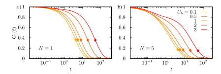
**FIG. 2.** Position autocorrelation function  $C_1(t)$  of an isolated particle (a) and the leftmost tagged-particle in a single file with five particles (b) as a function of the barrier height  $U_b$ . Symbols denote  $C_1(\Lambda_1^{-1})$ .
