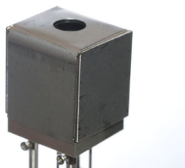
Figure 2.4: Photograph of a manometer head, covered by the protection cap with a hole which has a diameter of approximately 10 mm [17].
