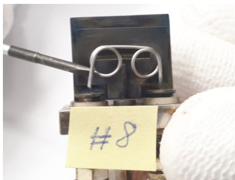
Figure 2.8: Example of a broken manometer from ASDEX Upgrade at the summer opening 2019, failure due to a partly disjointed filament [17].
