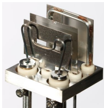
(a) Photograph of a pressure gauge [17].
