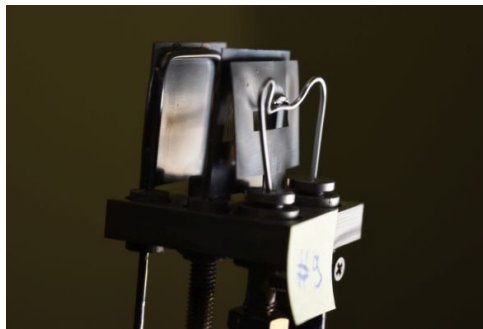
Figure 2.7: Example of a broken manometer from ASDEX Upgrade at the summer opening 2019, failure due to short circuit between the filament and the control electrode [17].
