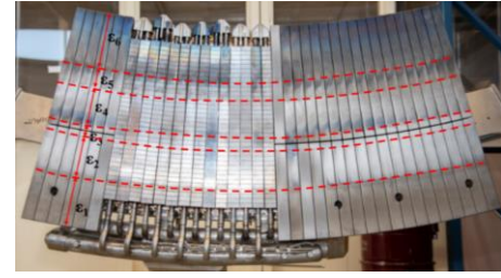
Fig. 2. Photography of the lower divertor sector and illustration of the piecewise constant profile constituted of six emissivities ( \varepsilon_1=0.2 , \varepsilon_2=0.07 , \varepsilon_3=0.1 , \varepsilon_4=0.07 , \varepsilon_5=0.15 and \varepsilon_6=0.3 [5])
