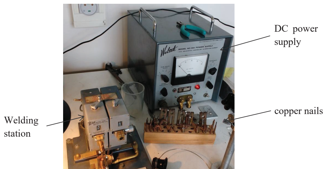
Figure 4.1 Photo of the spot-welding machine in S. T. Purcell group in Lyon, France
